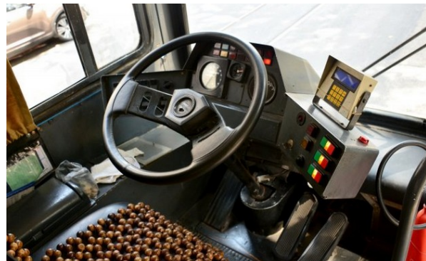
Painel de comando trólebus Mafersa 5307. ( https://onibusbrasil.com/diogoamorim/5369656?context=prefix )
